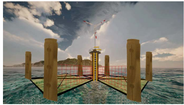
Modules and connecting nodes configured as MARLIN AQUA semi-submersible offshore fish farm
